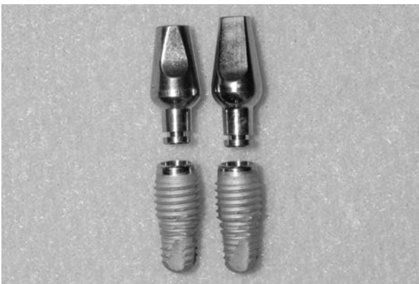
Fig. 1. Fixture and abutment used for this study (Left: conventional abutment, Right: FDI abutment).
