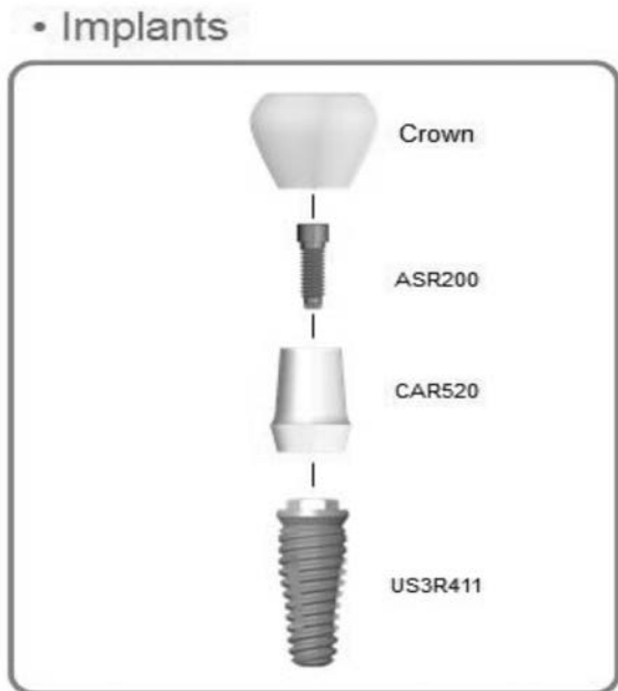
Fig. 1. The implant is composed of fixture (US3R411), abutment screw (ASR200), abutment (CAR520) and crown.
