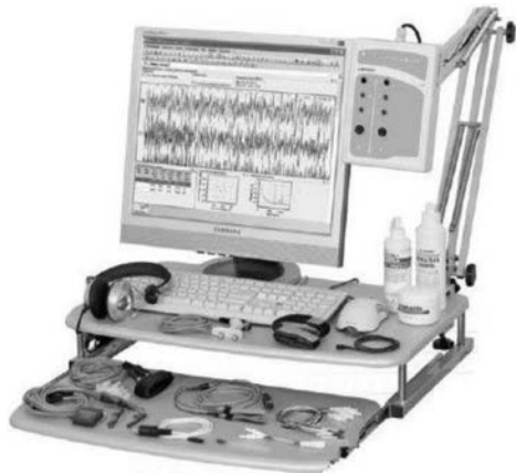
Fig. 1. Neuro-EMG-micro (Neurosoft™, Ivanovo, Russia) was used to quantify the threshold value, duration, delayed time, and amplitude of mental nerve blink reflex response.
