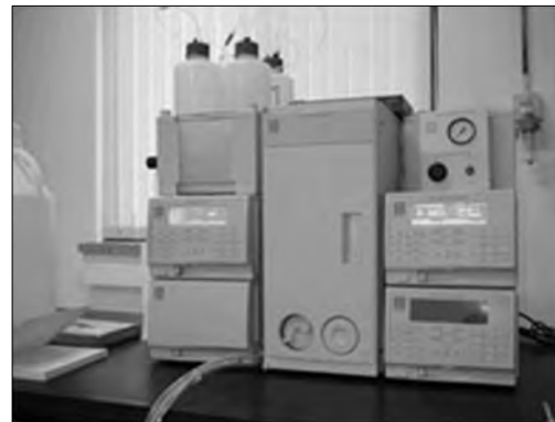
Fig. 4. Conjugated bases of HCl, HNO 3 were measured by Ion Chromatography System.
