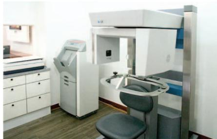
Fig 1. Cone Beam Computed Tomography System (i-CAT™, ISI, USA)
