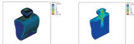
Fig. 7. Equivalent overall stress (Model 4, 30°, Point A).
