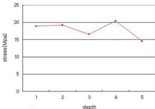
Fig. 13. Comparison of the stress according to the apical–coronal implant position in the bone (loading site = A, load = 90°).
