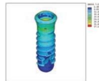
Fig. 8. Equivalent stress on the implant (Model 5, 90°, Point A).
