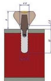
Fig. 3. Surface dimensions of the internal fixture.
