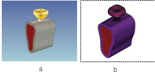
Fig. 2. 3-D geometry of the full body (a) and 3-D finite element model (b).
