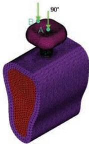
Fig. 5. Load owing to a 90° vertical force. Point A: the center of the pontic, Point B: buccal cusp
