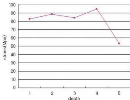
Fig. 12. Comparison of the von Mises stress according to the apical–coronal implant position in the bone (loading site = A, load = 30°).
