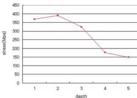
Fig. 16. Stress differences in the abutment screw (loading site = A, load = 30°).
