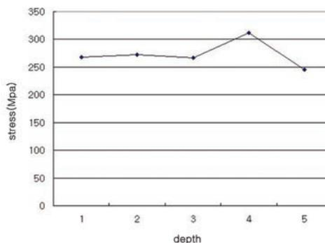
Fig. 15. Stress comparison for an internal screw (loading site = A, load = 90°).
