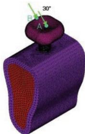
Fig. 6. Load owing to a 30° oblique force. Point A: the center of the pontic, Point B: buccal cusp
