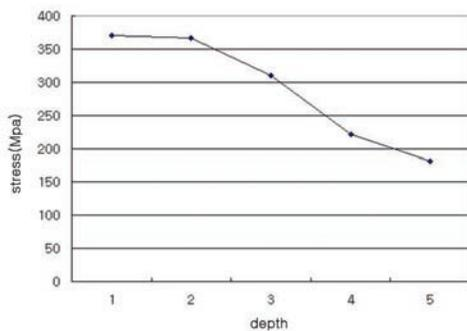
Fig 18. Von Mises stress in the implant (loading site = B, load = 90°).
