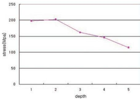
Fig. 17. Stress differences in the abutment screw (loading site = B, load = 30°).
