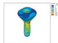
Fig. 10. Stress on each component (implant, abutment, and crown) (Model 4, 30°, Point A).
