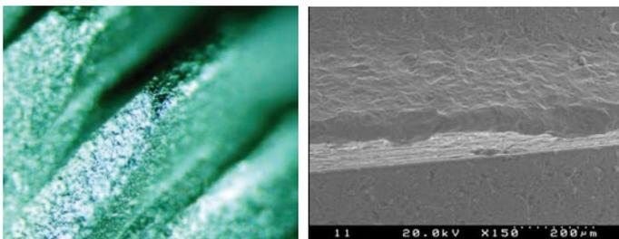
Fig 5. screw-type implant, dual acid etching surface (Frialit-2), evidence of milling
